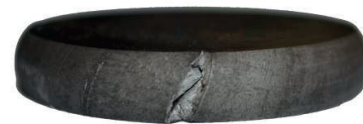
Fig. 10. A general view of a 20MnB4 steel specimen after the cold upsetting process with a relative strain of 75%
