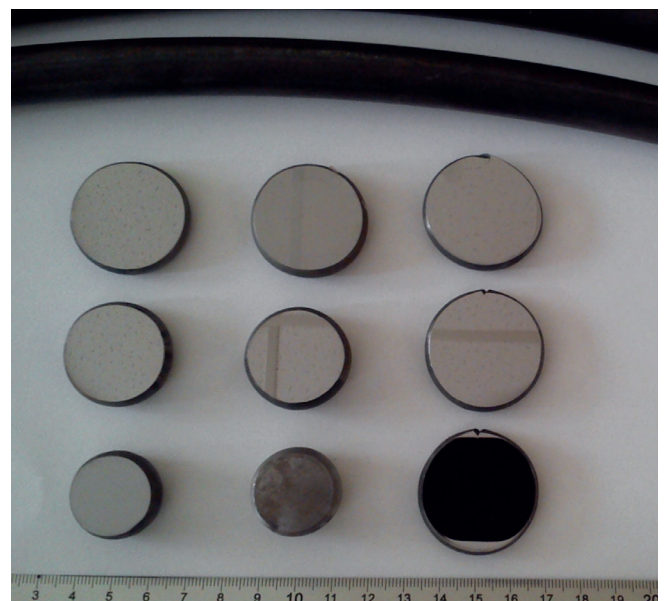
Fig. 1. 16.5 mm-diameter 20MnB4 steel wire rod and test specimen microsections
