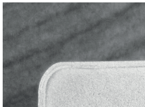
Fig. 3. Rim of coarse crystals formed during extrusion of MgAlZn alloys
