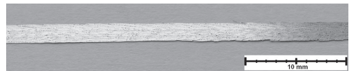
Fig. 4. Image of the AlSi11,6Mm4 alloy ribbon surface cast at a speed of 30 m/s, wheel-facing side
