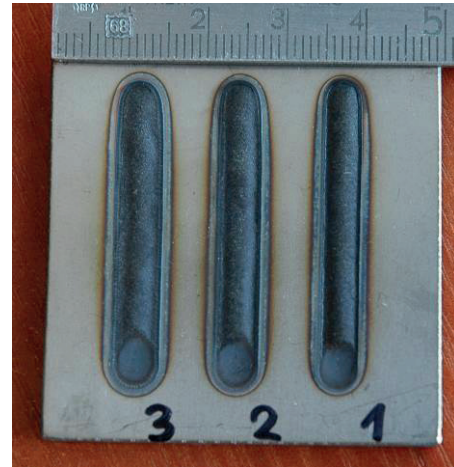
Fig. 4. A view of single stringer beads produced by defocused disk laser beam with a diameter of 6.8 mm on the substrate of stainless steel (bead width in a range of 6-6.5 mm)
