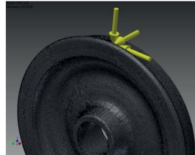
Fig. 8. Model mesh with applied forces for monoblock wheel 920 185a
