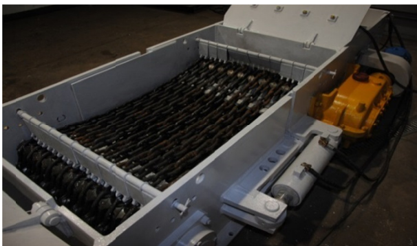
Fig. 3. Test rig, A – a view of the test chamber of the test rig during the wear tests with dry quartz abrasive (variant 1), B – a view of the test chamber of the test rig during the wear tests with dry quartz abrasive and a dynamic load (variant 2); the arrow indicates the installed beaters
