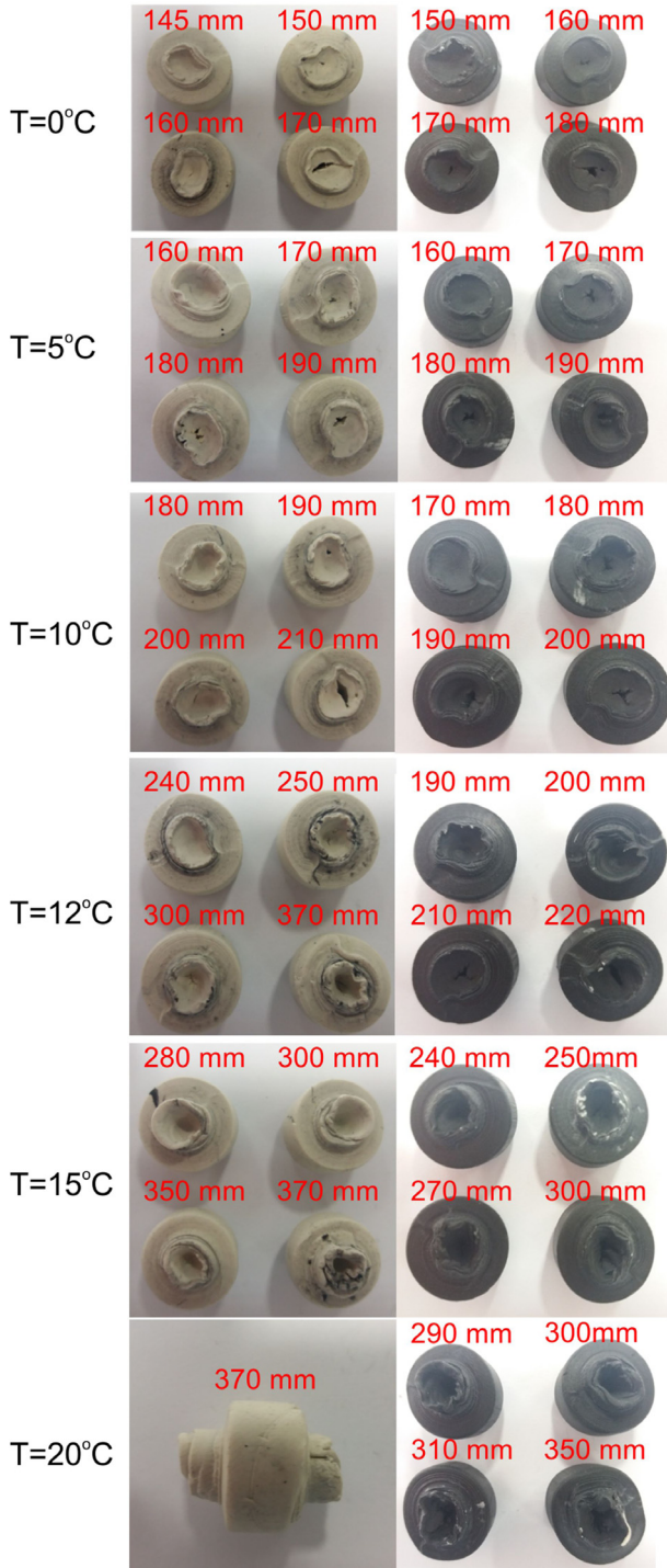
Fig. 5. Samples of the material model after rotary compression test (RTC)
