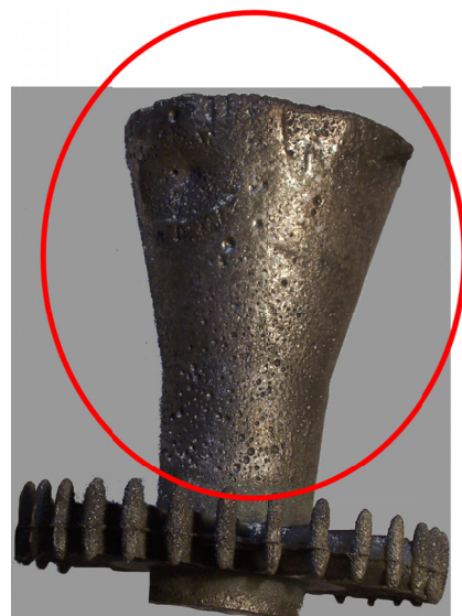
Fig. 3. A view of an exemplary gravity cast with marked massive sinkhead
