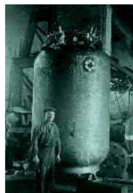
Fig. 1. Protocol from 1930 describing the study of duplex stainless steel grade 453S with 25% Cr, 1.5% Mo (left side), gunpowder reactor of the same steel grade supplied to a Belgian factory in 1933 (right side) [11]
