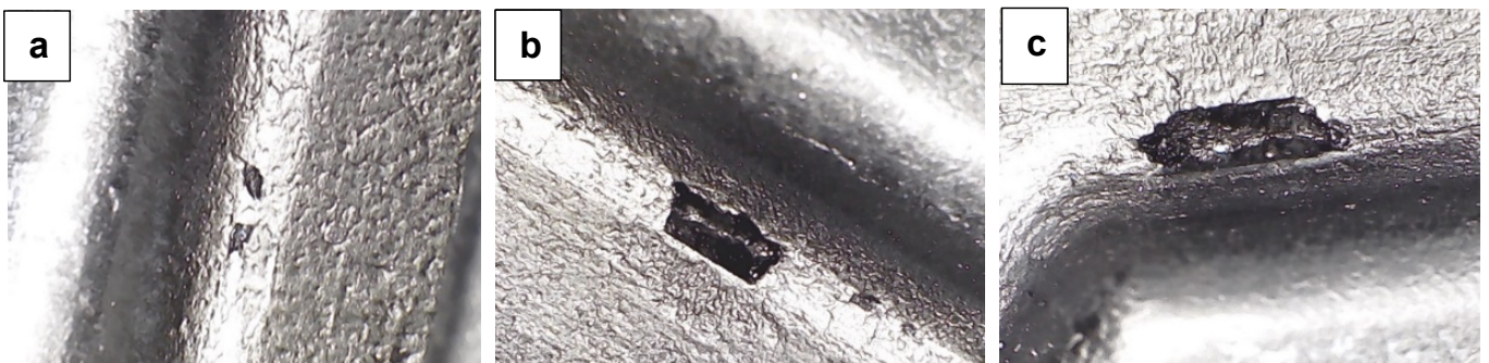
Fig. 3. Images documenting small (a) medium (b) and large (c) chipping damage to the pin surface after 19 500 injections (please note cracks spreading from the latter one)
