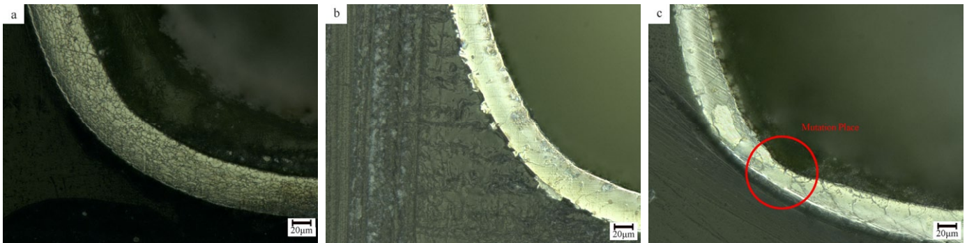
Fig. 14. Microstructure at the rounded corner of the drawing cup: (a) 950°C, (b) 1050°C, (c) 1100°C
