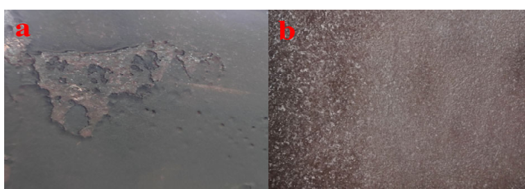
Fig. 5. Images of low arsenic anode passivation, 65°C, at current density of 250 A/m 2 (a) and normal anode dissolution, 65°C, at current density of 300 A/m 2 (b) respectively
