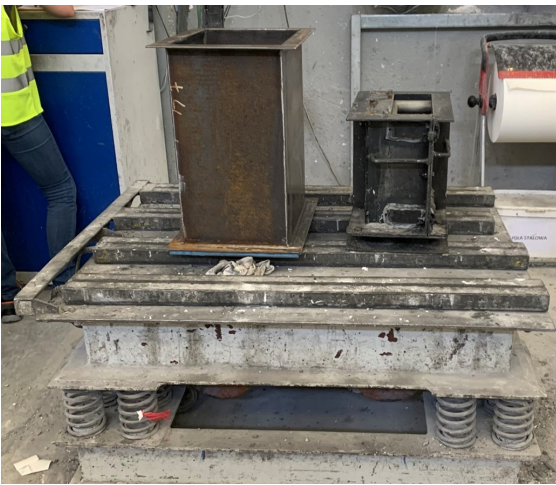
Fig. 1. Moulds on the vibrating table
