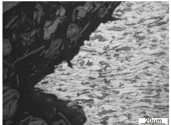
Fig. 8. Light microscope image of fracture after tensile test
